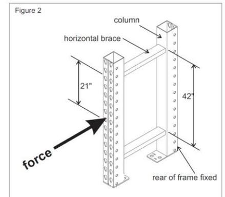
The industry standard, open-back (roll-formed) frame assembly failed at 3,200# of pressure. When subjected to a similar 3,200# load, the SK2000 assembly exhibited no deflection, nor any visually detectable damage. The SK2000 frame assembly continued to withstand increasingly heavy amounts of pressure, until reaching its own yield point of 4,700# (See Figure 3).
