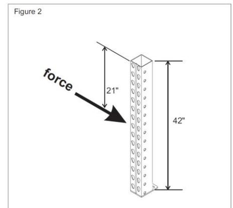
The industry standard, open-back (roll-formed) column failed at 1,900# of pressure. When subjected to a similar 1,900# load, the SK2000 closed tubular column exhibited no visually detectable damage. The SK2000 column continued to withstand increasingly heavy amounts of pressure, until reaching its own yield point of 3,200# (See Figure 3).
